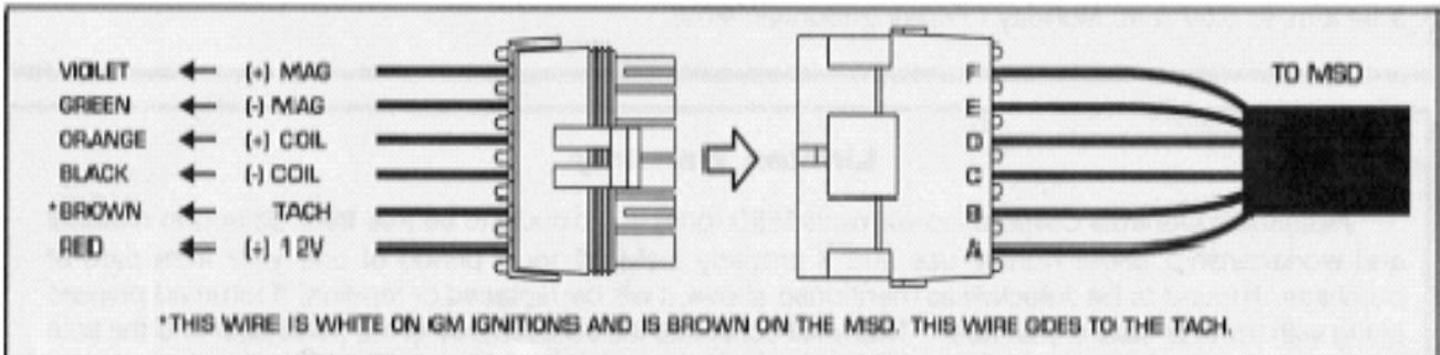
Above shows wiring order for connector installation on MSD 6AL and 6T Ignition Box
