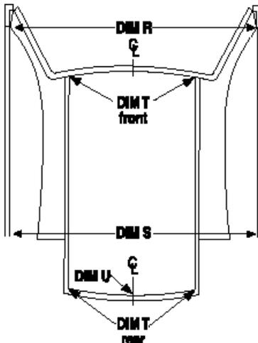
This drawing shows roof corner dimensions to help you properly locate the roof. Once the roof is located, confirm that highest point on the roof (Dim. H) is 47". This dimension is measured 10" back from the windshield.
